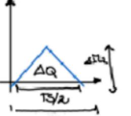
$$\begin{cases} \Delta Q = C_2 \cdot \Delta v_0 \\ \Delta Q = \frac{1}{2} \cdot \frac{T_s}{2} \cdot \frac{\Delta I_{L2}}{2} = \frac{T_s \cdot \Delta I_{L2}}{8} \end{cases}$$
