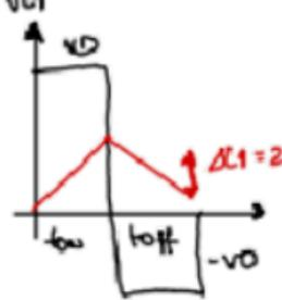
$$v_{L1} = L \cdot \frac{\Delta I_1}{\Delta t} = v_0 = L \cdot \frac{\Delta I_1}{t_{on}}$$
