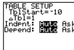
Press **ENTER** to select **Indpnt: Auto** (automatically generated independent values). Press  $\downarrow$  **ENTER** to select **Depend: Auto** (automatically generated dependent values).
