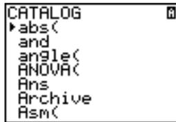
2. Press **[↓]** or **[↑]** to scroll the **CATALOG** until the selection cursor points to the **GarbageCollect** command or press **G** to skip to the commands starting with the letter **G**.
